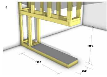
Build the chimney framework with consideration to flue pathways and meet the minimum fireplace opening requirements (850mm H x 1320mm W x 350mm D). Ensure a continuous base for the fireplace.
